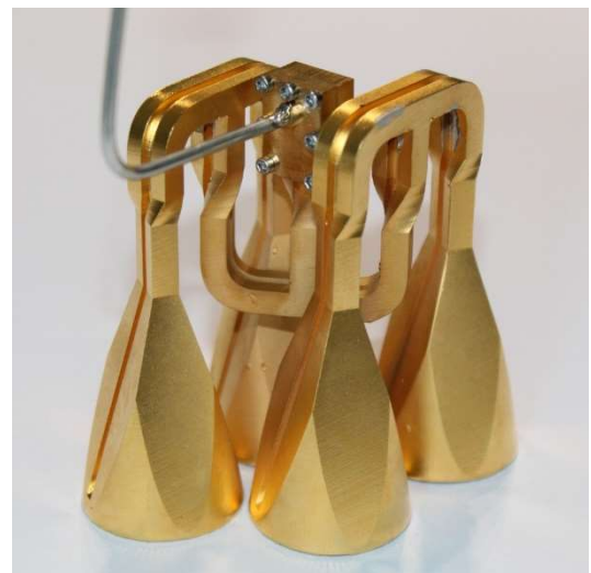
Prototype of a monopulse horn antenna with feed network, manufactured using 3D printing technology and metal-coated by electroplating
