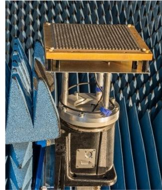
The antenna (with and without the radome absorber) in the chamber
