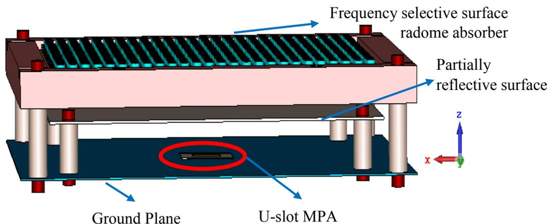
The layout of the antenna and radome integration
