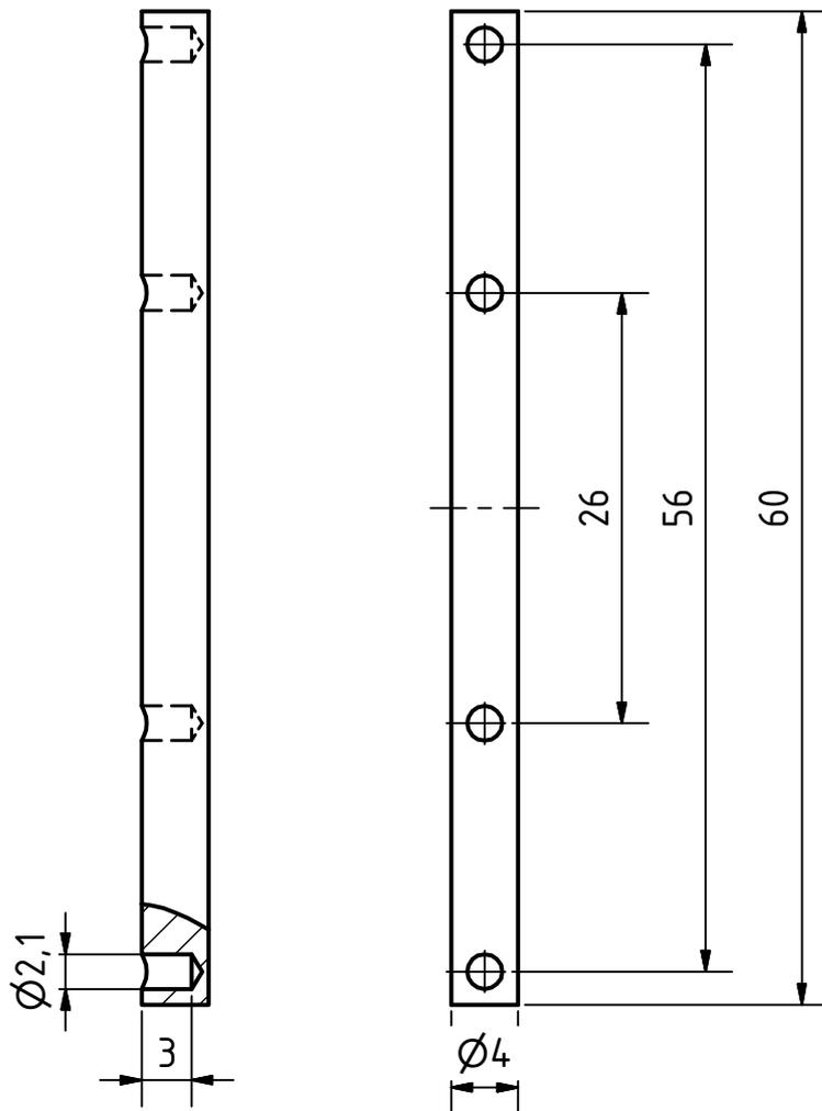
4X Messingdraht  $\varnothing 2$  98mm lang
