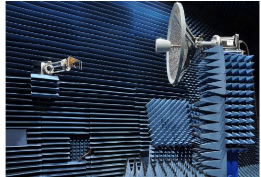
Spherical Near-Field Measurement Chamber of the IHf
